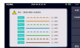
Network Cable Test
